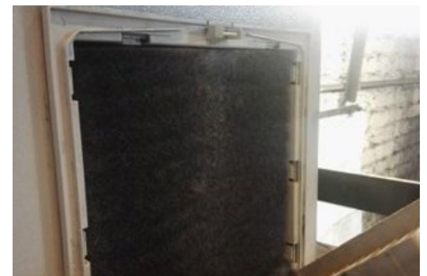
Fig. 4 Field test with a chopped-fiber filter
